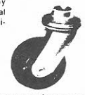
Pipe base swivel casters available with 3/4" to 8" wheels for 400-750 lbs. capacity; 1" pipe threads standard; other sizes available if quantity warrants.
