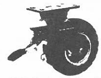
Cam-action foot brake with PVC-coated shoe directly contacts wheel tread; particularly effective with diameters 8" and larger.
