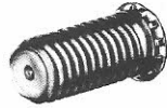
Self-clinching Stud — thread sizes #2 thru 3/8" & M3 thru M8, minimum 0.040" metal thickness & lengths to 1 1/2".
